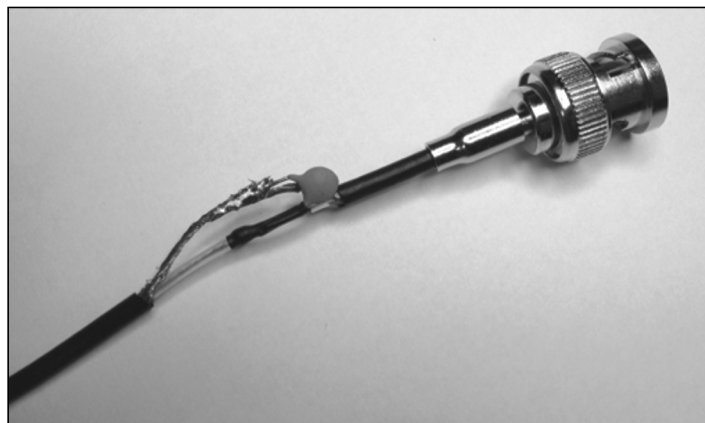
Figure 11—Installation of the shunt capacitor.
